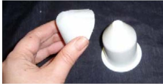
Keep in mind that the material takes a little while to set, so you may want to hold it in place until it hardens enough that it won't deform. Applying cold water will speed the setting. Interacting with the Wonderflex is a simple matter of dealing with temperature rather than waiting for a chemical reaction.
