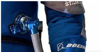
Airflow diverter vent keeps astronaut cool. Photo: Boeing.
