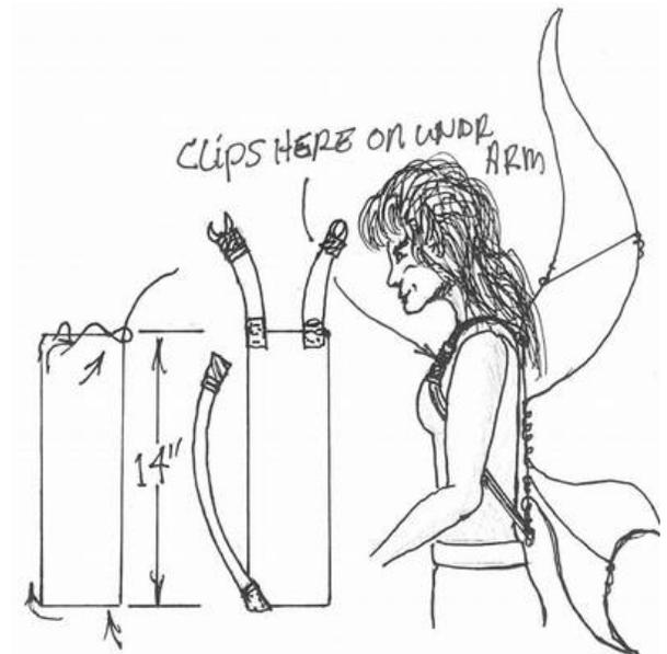
To make the wings easier to take on and off and to adjust, we supplied parachute clips. The students cut shorter lengths of webbing that attached to the top of the frame and to one half of the clip, and a longer lengths of webbing that attached to the bottom of the frame and to the other half of the clip. They left enough extra strap to adjust the length once the clips were closed.
