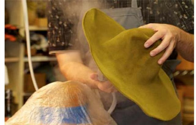
3. Steaming felt blank softens the felt to stretch and form.
