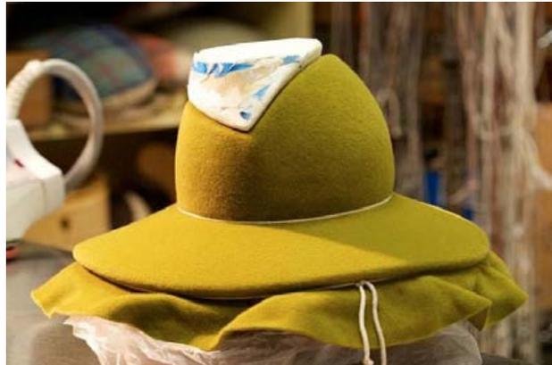
8. Recessing tool pressed into form to shape the crown.
