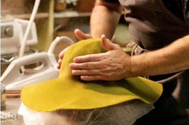
4. Quickly shape the hot felt over the block.
