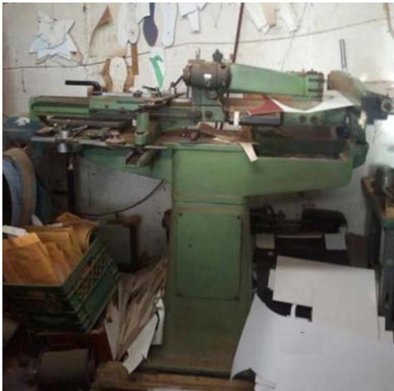
Grading machine cuts patterns from masonite master.
