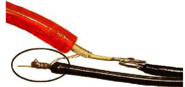
Soldering EL wire to driver and power supply. Photo courtesy [CoolNeon.com](http://CoolNeon.com).
